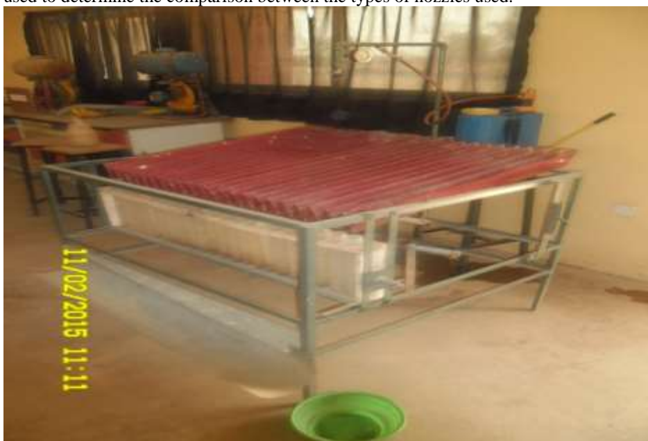
Plate 1: Patternator used in determining the spray volume distribution pattern of the sprayer nozzle at various height and pressure.
